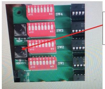
Turn off the machine normally, use hand to press the "service" button and do not release the finger, simultaneously turn on the machine, after 5 seconds, release the finger.
