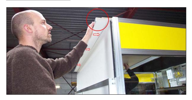
• Slide the front roof-panel into the crane until it lies in the right position.
